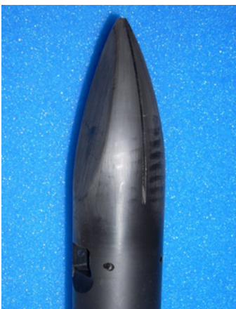
We produced just two of these parts, used to apply labels to small bottles in a dairy plant.
