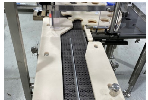
These packaging lines include Slideways belt attachments, guide blocks and pin guides.
