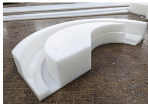
These packaging lines include Slideways belt attachments, guide blocks and pin guides.
