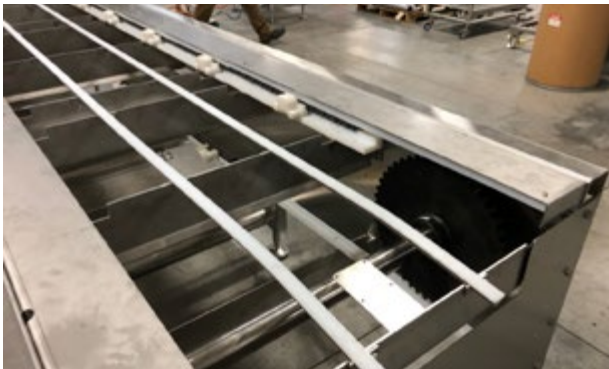
OEM conveyor builder in Wisconsin building bakery system that uses UHMW belt supports, pusher blocks, pusher support, return guide, and stainless steel levelers.
